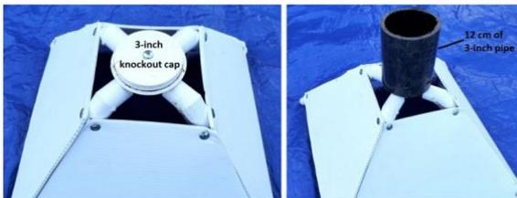
Left: A 3-inch knockout cap screwed onto the top of the tent. Right: A 12 cm length of 3-inch pipe attached to the knockout cap.
