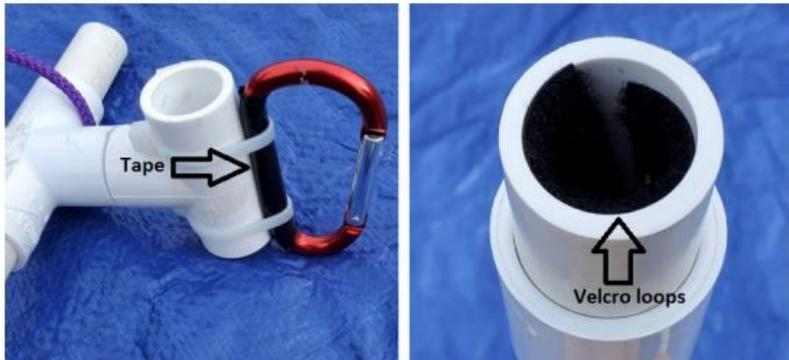
Left: [3" aluminum carabiner](#) on the mooring connector. Three layers of tape on each side of the carabiner will prevent it from rolling against the 1/2-inch tee when secured with cable ties. Right: Velcro loops inside the 1-inch PVC coupling.
