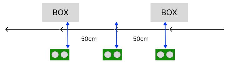
The boxes move one by one from right to left, at a distance of 50 cm from the sensors. There are only 3 distance sensors. The box cannot appear or disappear in the middle of the conveyor.
